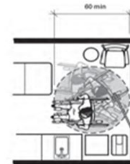
Plan view of part of an examination room showing clear floor space for turning a wheelchair. This space can also make it possible for use of a portable patient lift.
