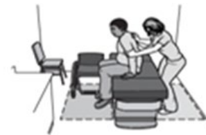
Patient sitting on adjustable height exam table positioned with clear floor space on both sides
